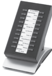
Add-On Module 20 programmable buttons KM5020
